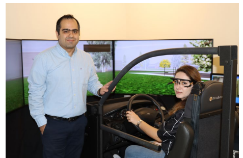
UAS-induced driver distraction experiments using a driving simulator and eye-tracker by Dr. Reza Akhavian and graduate student Newsha Emaminejad.
